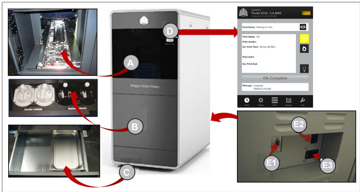
The three dimensional solid parts built by the printer consist of two materials (support material and part material). The support material is a wax based material providing adhesion to build platform, as well as, providing material used to produce supports required to build the model.
