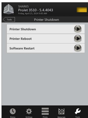
**Printer Shutdown:** Click on the arrow key to shutdown printer. Click the arrow keys to reboot printer or to restart the software.
