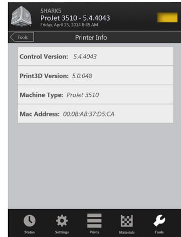
**Printer Info:** provides information about the control software version, Print3D software version, machine type and its address.
