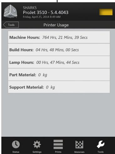
**Printer Usage:** provides printer usage information in hrs, mins, & secs. and how much material has been used.
